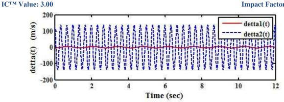
Figure.4 Undamped Modal response of  $\dot{\eta}$
