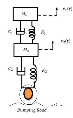
Figure.2. Mathematical model of quarter car suspension system
