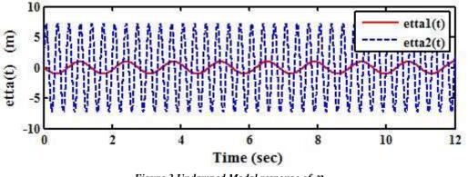
Figure.3 Undamped Modal response of  $\eta$
